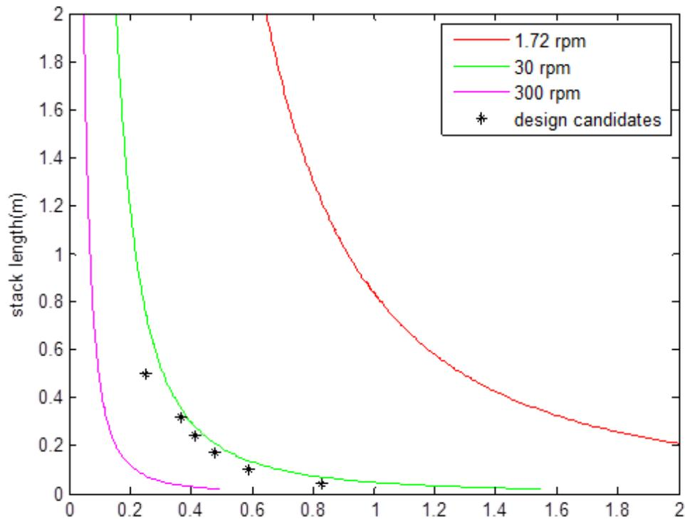
**Figure 9. 10kW generator sizing with different aspect ratio**
