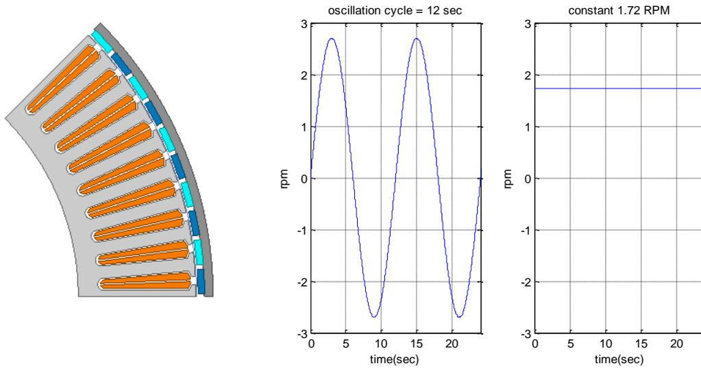
**Figure 5. Geometry and speed for constant vs oscillation calculations**
