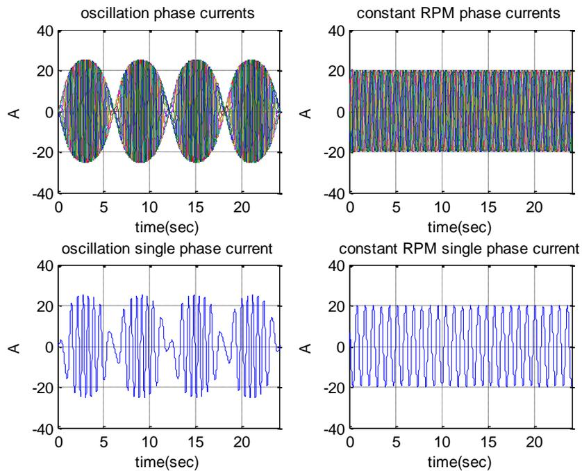
**Figure 6. Generator phase current for sinusoidal oscillation (left) and constant speed (right)**
