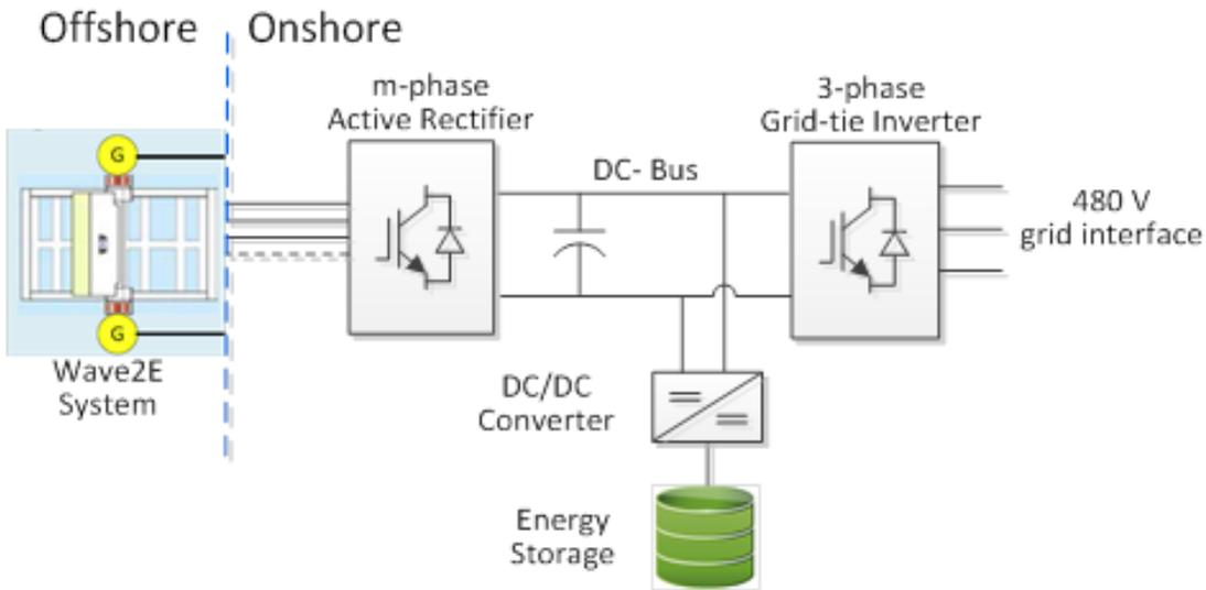
**Figure 4 . Electrical PTO system configuration**
