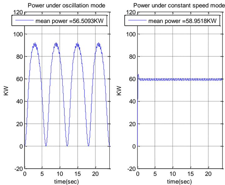
**Figure 8. Generator output power for sinusoidal oscillation (left) and constant speed (right)**
