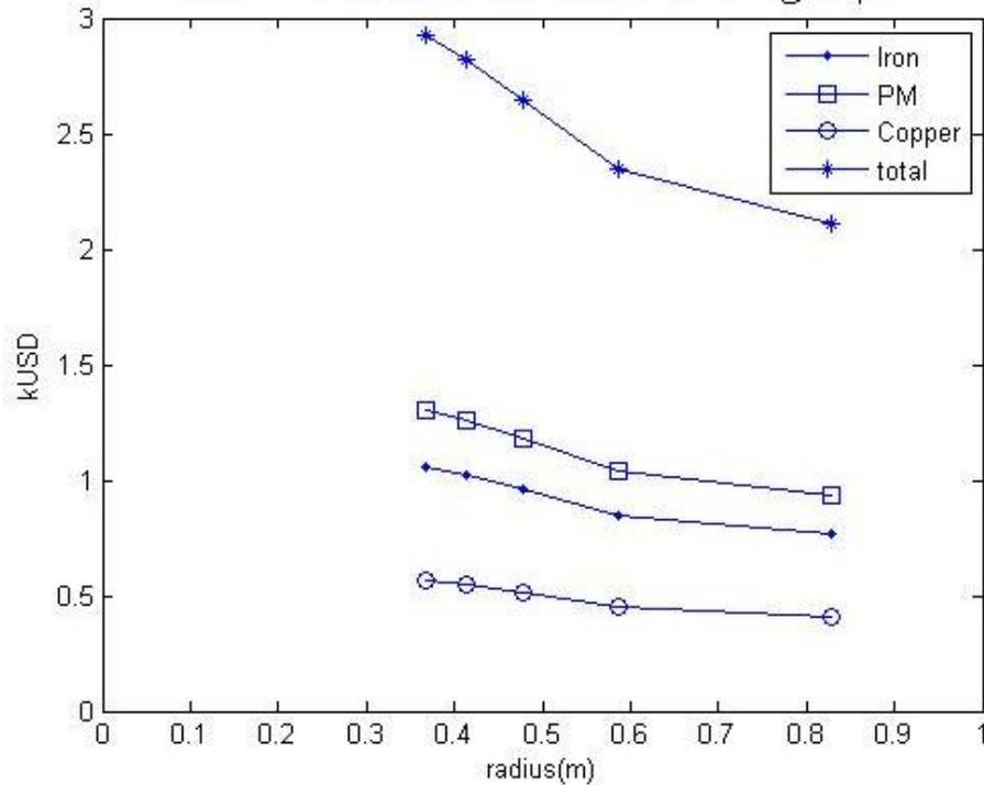
Figure 10. Active material cost estimation of 10 kW, 30 rpm FEA models
