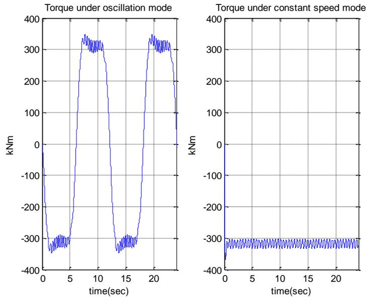
**Figure 7. Generator torque for sinusoidal oscillation (left) and constant speed (right)**
