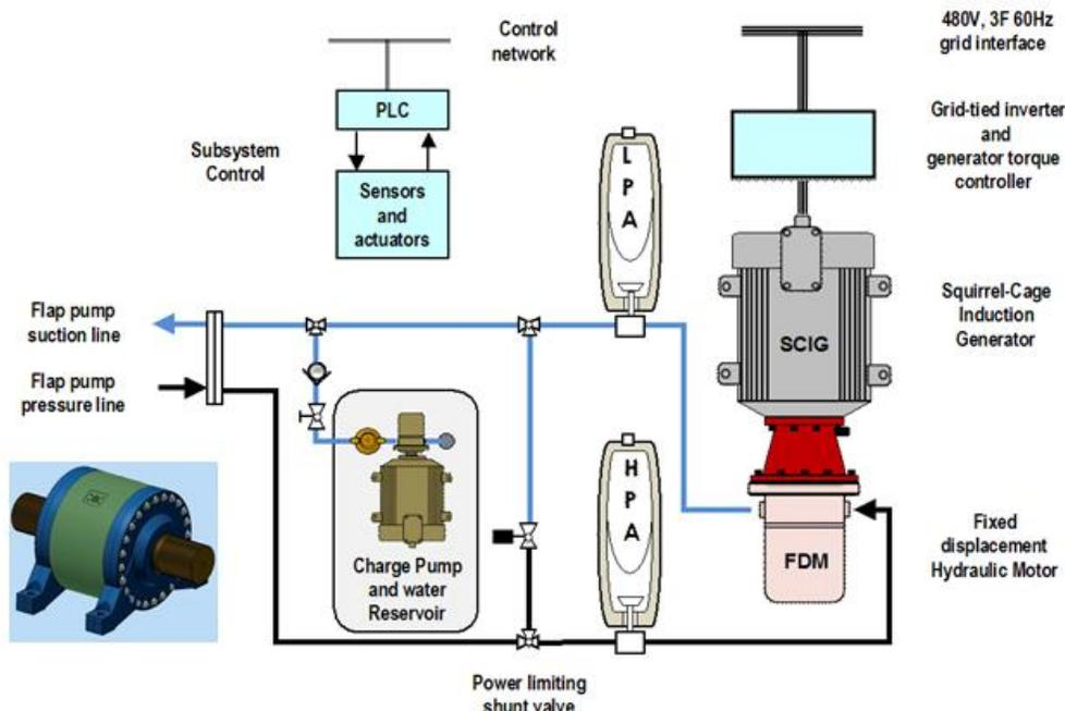
Figure 3. Reference hydraulic PTO system solution
